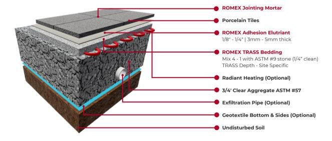
This innovative and permeable bonded system allows water to flow right through and back into the ground preventing any freezing. This durable build can also withstand vehicle weight upwards of 40T and prevents surface movement from occurring.
