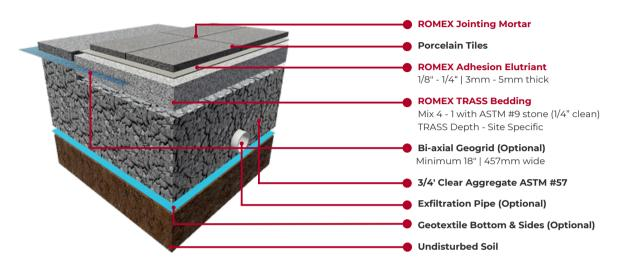
ROMEX bonded edge system only requires the perimeter tiles to be bonded with TRASS while the interior tiles will be bonded to the open graded base, using ADHESION ELUTRIANT to prevent any lateral movement on the inside.
