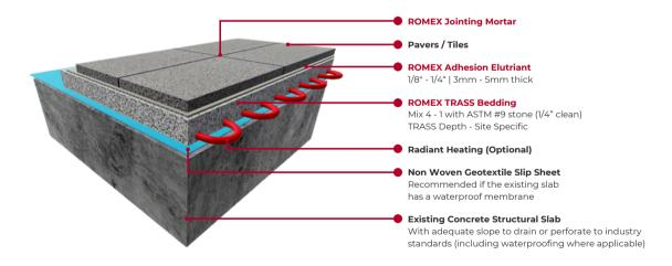
This unique system is perfect for rooftop applications and helps eliminate wind uplift liability. Our tile bedding at 1.5" | 38mm depth is only 14lbs | 6.3kg per square foot, making this an extremely lightweight bonded build.
