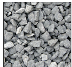
ASTM Stone #57 (3/4" clean & dry angular stone)
